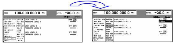
Execute the calibrations from the menu UTILITIES/CALIB/ALL. The generator should be in a warmed-up condition (at least 30 minutes switched on). After the calibration all errors will disappear.
